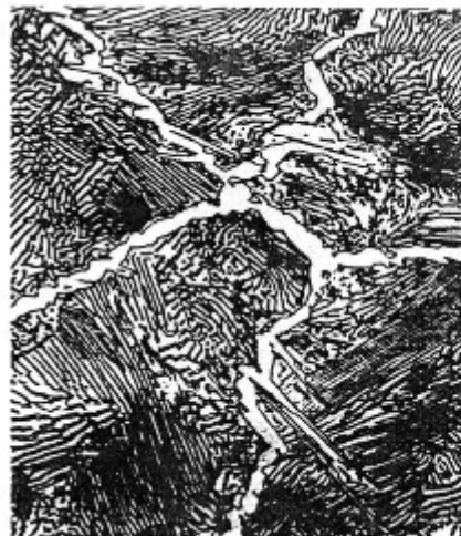
FIGURE 9.31 Photomicrograph of a 1.4 wt% C steel having a microstructure consisting of a white proeutectoid cementite network surrounding the pearlite colonies. 1000 \times . (Copyright 1971 by United States Steel Corporation.)
